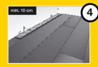
The width of last row should be more or equal 10cm. If so, cut the width of the first row to be installed. If the distance between the wall (minus dilation gap) and the last row is
