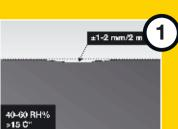
Relative humidity between 40 and 60% and temperature minimum 15C° must be ensured during laying and use. The subfloor flatness tolerance should be max. 2 mm/meter.
